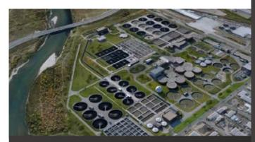
The 36-MGD Bonnybrook WWTP in Alberta, Canada was delivered by Stantec using the Construction Manager at Risk (CMAR) alternative delivery method.
