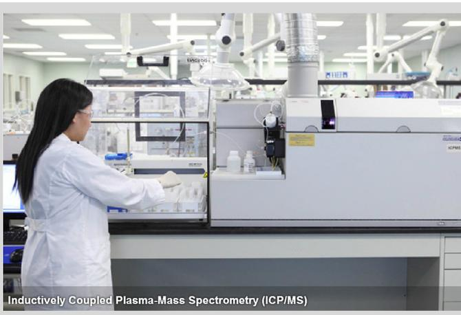
Inductively Coupled Plasma-Mass Spectrometry (ICP/MS)
