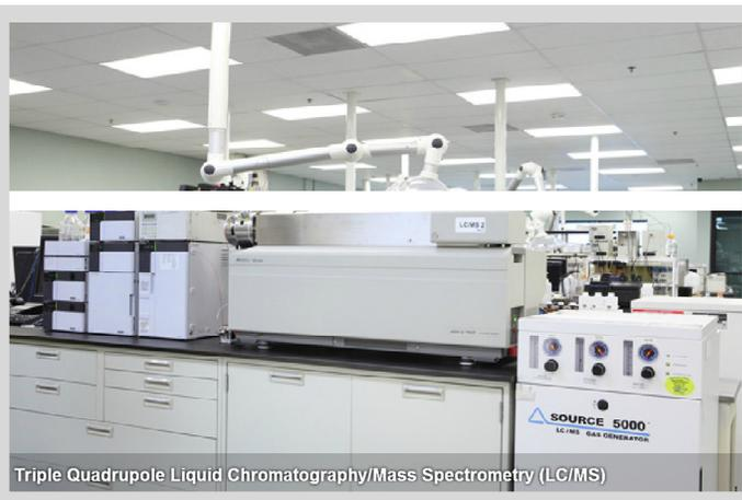
Triple Quadrupole Liquid Chromatography/Mass Spectrometry (LC/MS)
