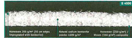
Bentofix® cross-section used in Dam Sainte-Marguerite
